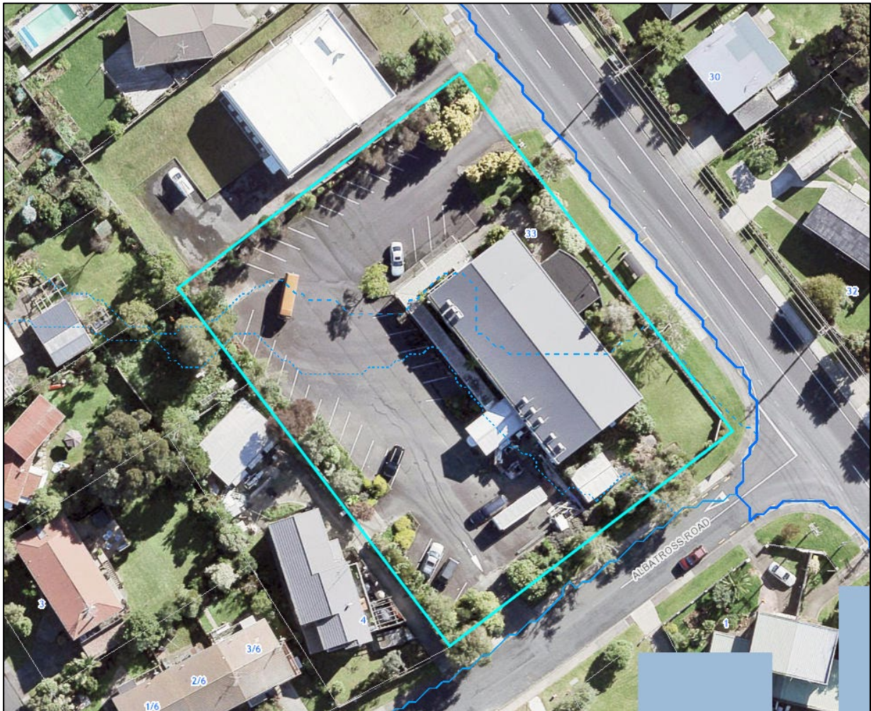
Figure 7: Images showing the two minor overland flow paths on the application site.
